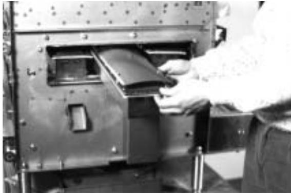
16. Remove the Upper Disposable Burners and clean as follows:
