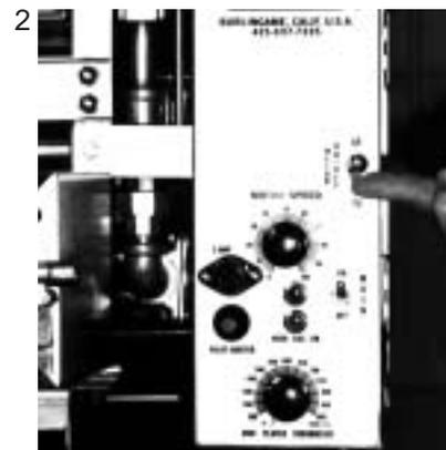
3. Set Motor Speed Control knob to desired setting.
