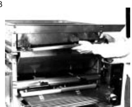
4. Remove the Upper Disposable Burner Front Reflector, and clean with soap and water.
