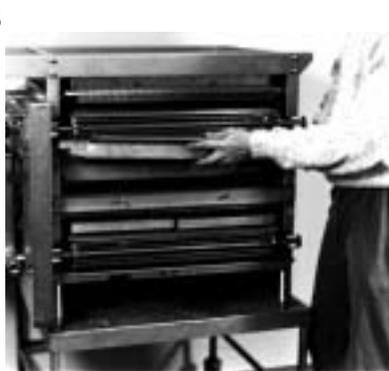
14. Remove the Lower Burner Reflector. Notice the position of the piece before removing it, so that you can re-install it properly. Clean by soaking in soap and water.
