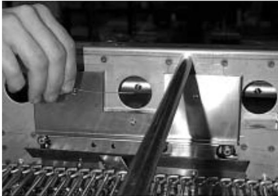
**CAUTION: NEVER CLEAN BURNER ORIFICES WITH ANYTHING OTHER THAN THE APPROVED BRUSH, (ie. PAPER CLIP, TOOTHPICK etc...) AS THE ORIFICE WILL BE DAMAGED. THIS WILL CAUSE IMPROPER BURNER OPERATION AND WILL AFFECT THE PERFORMANCE OF YOUR BROILER.**
