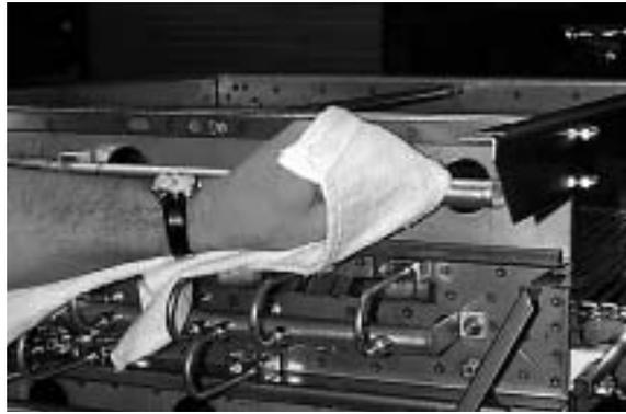
19. Using the Orifice Brush, carefully clean ALL orifices.
