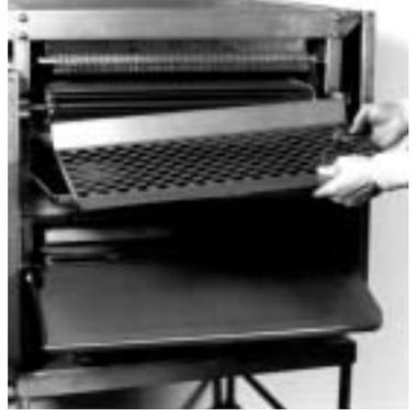
13. Remove the Stripper Blade (Doctor Blade). Scrape any built up residue from the blade. Clean by soaking in soap and water. Sanitize.
