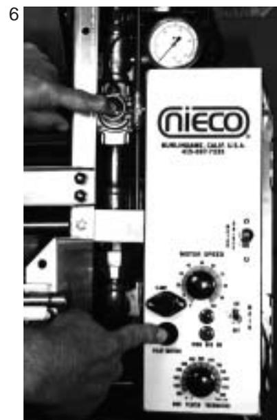
7. After lighting the broiler, check the gas pressure to be sure it is adjusted to the levels stated on the machine rating plate. Allow the broiler at least 40 minutes to warm up.
