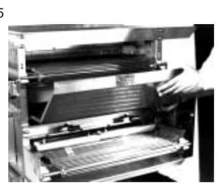
5. Remove the Grease Pan by sliding it out the front. Clean daily using soap and water.
