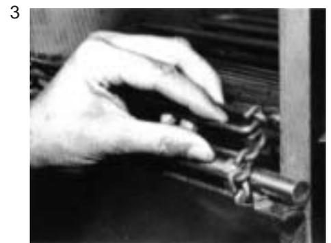
To reassemble, reverse the procedure. Be sure to reassemble the belt with the knuckle opening facing away from the direction of travel.
